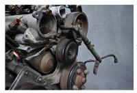
STEP 1: REMOVE THE DRIVE BELT TO GAIN FULL ACCESS TO THE PULLEY SYSTEM.
