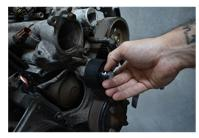
STEP 5: WITH THE INSERT REMOVED PLACE THE NEW SMOOTH PULLEY ONTO THE MOUNTING BOSS AND SCREW IN THE SUPPLIED M10 BOLT BY HAND. IT IS ADVISED THAT YOU USE SOME LOW / MEDIUM STRENGTH THREAD LOCKER ON THE NEW BOLT.
