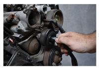
STEP 2: USING A 12MM SOCKET REMOVE THE BOLT THAT IS SECURING THE UPPER RIBBED PULLEY TO THE BLOCK.
