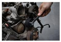
STEP 6: USING A RING SPANNER FIRMLY NIP UP THE BOLT. DO NOT OVERTIGHTEN OR YOU RISK STRIPPING THE THREADS OUT OF THE BLOCK.
